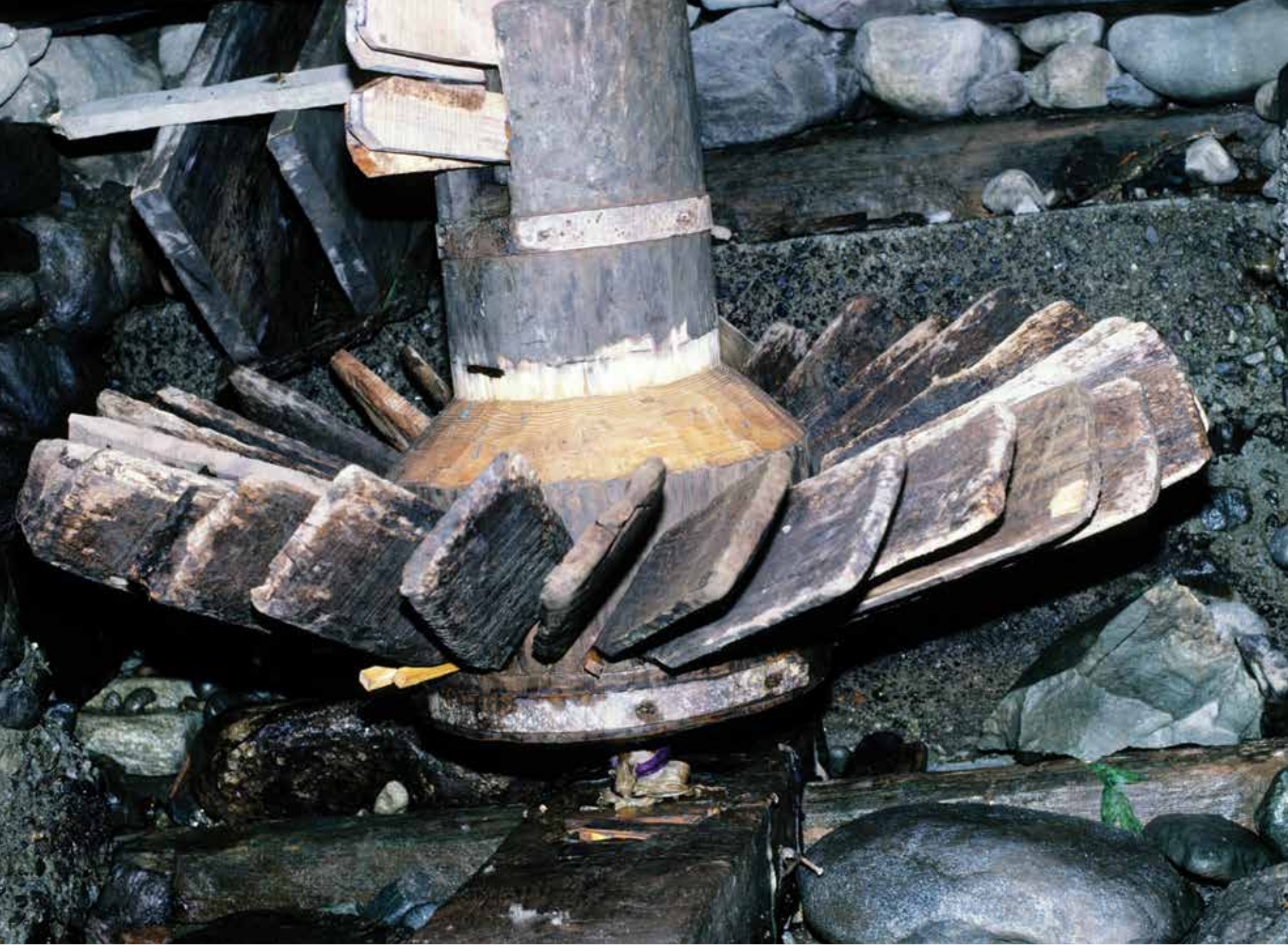
A wooden waterwheel used to turn a millstone for grinding corn. 1986.
