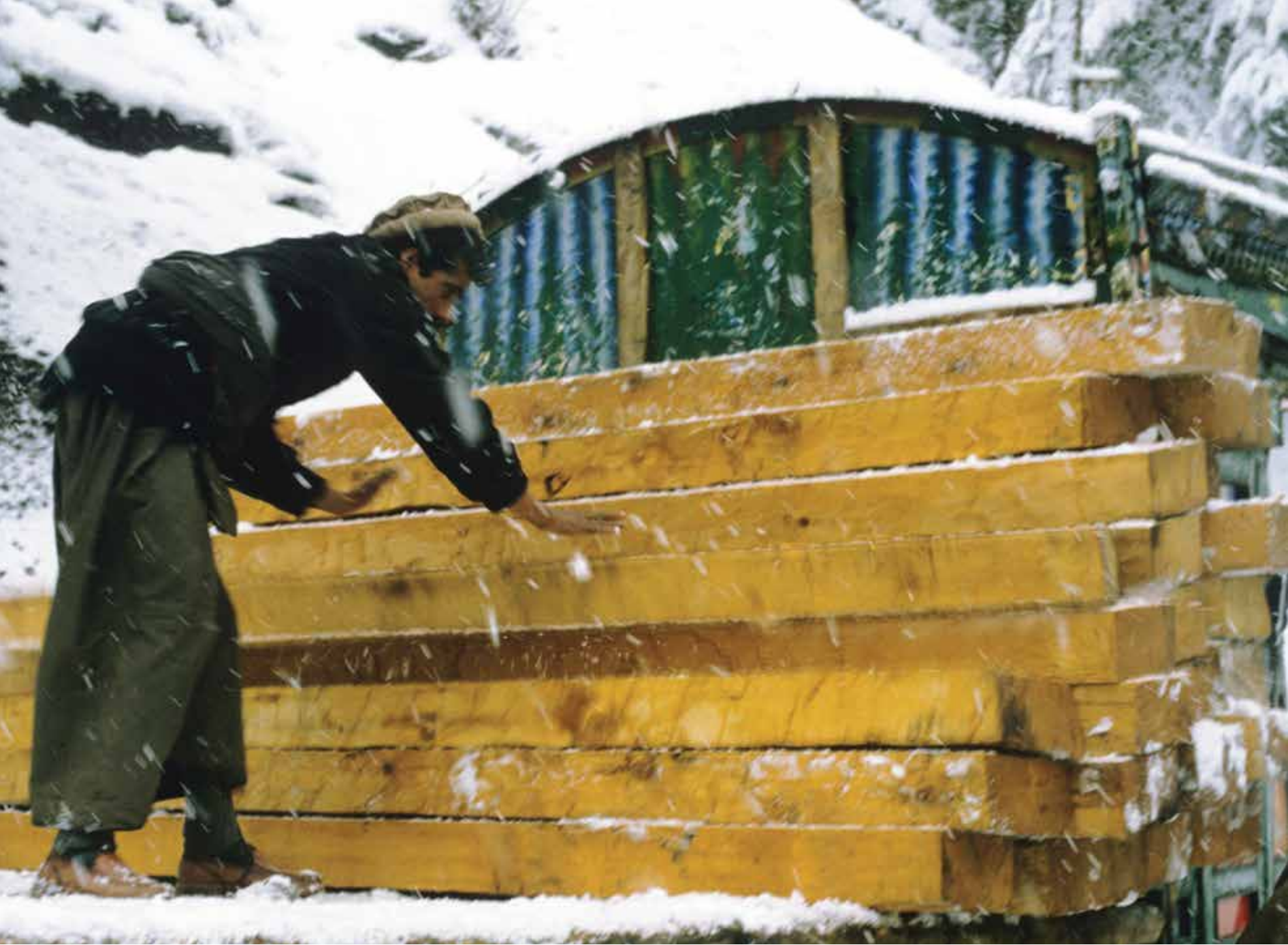
Timber sleepers could be transported easily by a man and were therefore produced directly in the forest after felling the tree. 1985.
